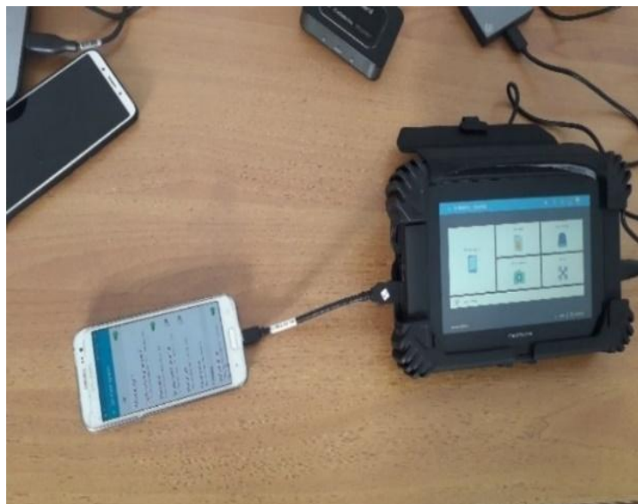
Figure 13 Connecting the Smartphone to Cellebrite's UFED Touch2
